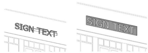
FIGURE 20-B: RACEWAY CABINET EXAMPLES
